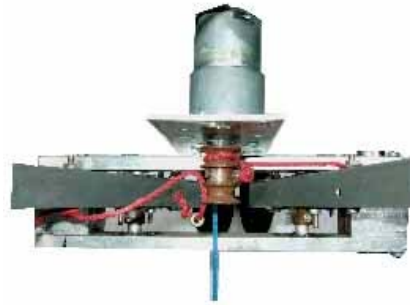
Figure 2.7 Gripper motor close view
